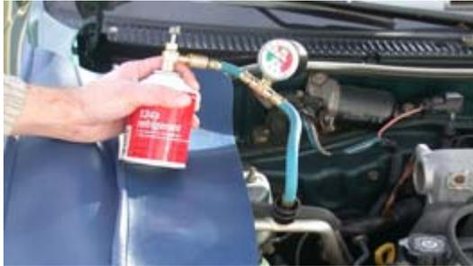
If the compressor does engage and the pressure exceeds 65 psi, the system is either overcharged with refrigerant or it needs other repairs. If this is the case, seek the help of a professional service technician.
